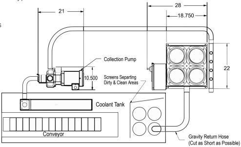
The Purge includes four quick change 5µm filter bags. The system is designed to accept most #2 filter bags/baskets. For general machining applications, use standard felt bags. If long-term use with fine debris is required used pleated paper bags.
