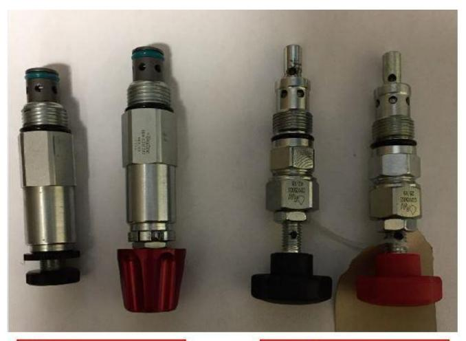
Parker Style Red Handle: HV RELIEF VALVE 100-100 PSI (water pumps) Black Handle: HV RELIEF VALVE 500-2000 PSI (oil pumps) Hydroven Style Black Handle: HV RELIEF VALVE 250-1250 PSI H (water pumps) Red Handle: HV RELIEF VALVE 500-2000 PSI H (oil pumps)
